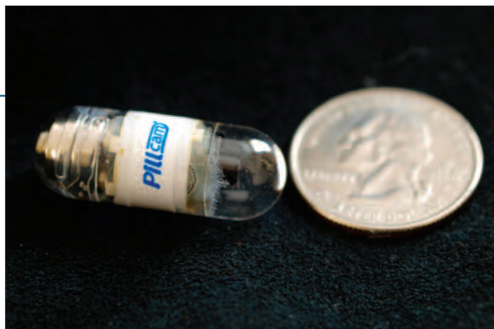
The new maneuverable wireless capsule is just about the size of a quarter.
